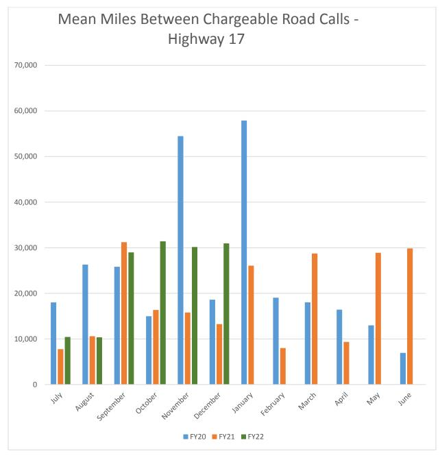
Above is the metric for mean miles between chargeable road calls for METRO's Highway 17 commuter route. Commuter buses tend to perform better due to more highway miles, fewer stops, and the newer fleet which has less wear and tear.
